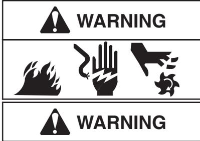
If you perform any maintenance on the engine, first disconnect the spark plug wire from the spark plug, and disconnect the battery at the negative terminal (electric starter engines only) to prevent unintentional sparking. Unintentional sparking can result in fire or electric shock. Unintentional start-up can result in entanglement, traumatic amputation or laceration. Use only correct tools.
