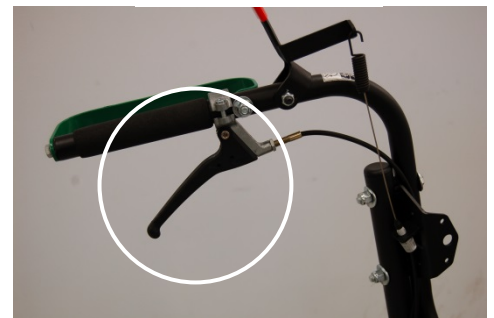
Fig. 7 Reverse Drive Lever
